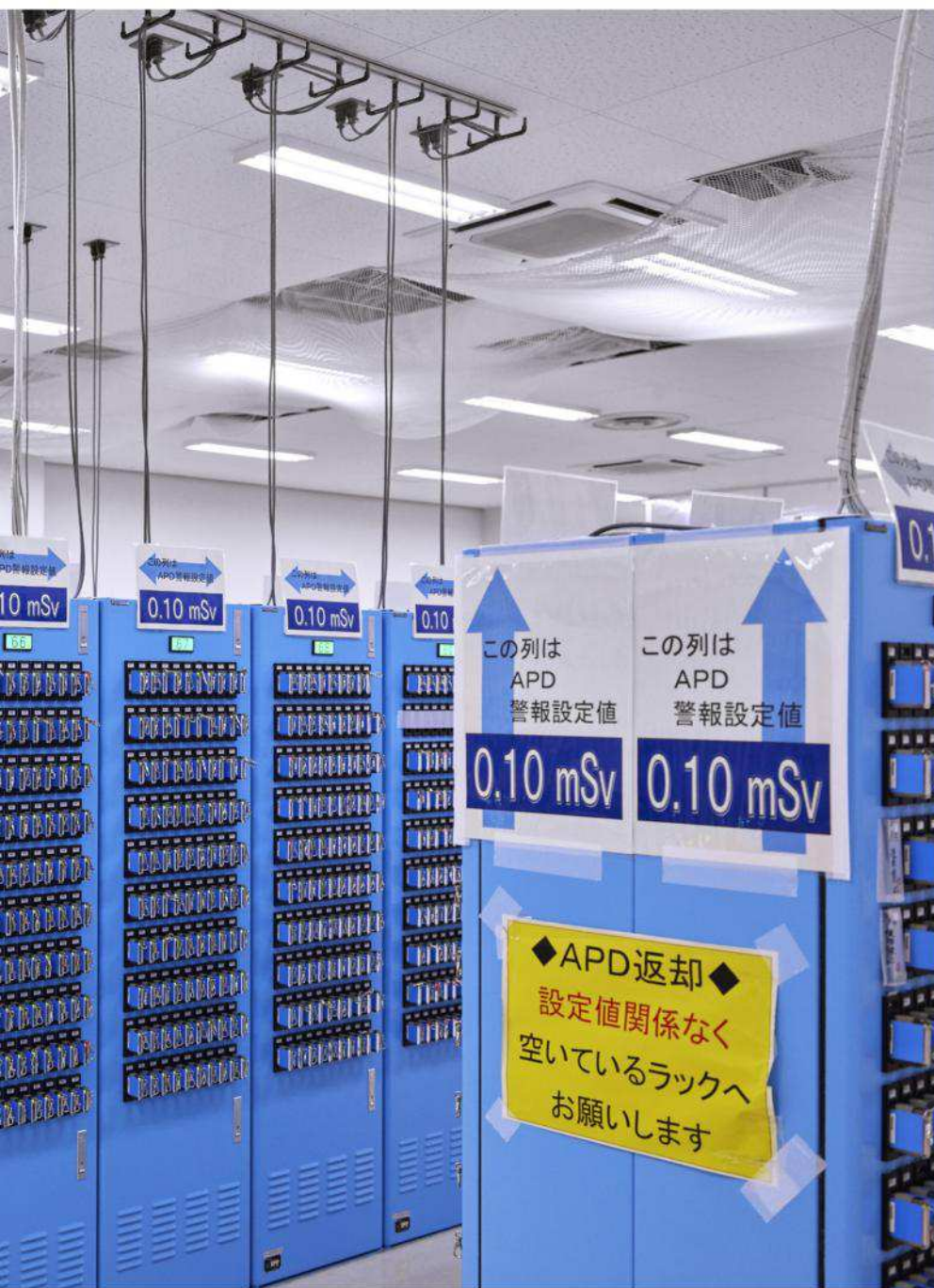
A ROBOT UNDERGOES TESTING AT THE GOVERNMENT’S NEW $100 MILLION R&D CENTER NEAR THE NUCLEAR PLANT [FAR LEFT]. INSIDE THE FUKUSHIMA PLANT, EACH OF THESE BLUE TOWERS [MIDDLE] HOLDS 100 PERSONAL RADIATION DETECTORS. KENJI MATSUZAKI [BELOW], THE LEAD SCIENTIST BEHIND LITTLE SUNFISH.
